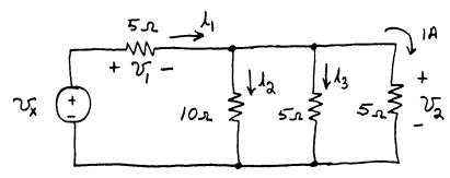
Applying Ohm's law, we have  $v_2 = (5 \Omega) \times (1 A) = 5 V$ . However,  $v_2$  is the voltage across all three resistors that are in parallel. Thus,
