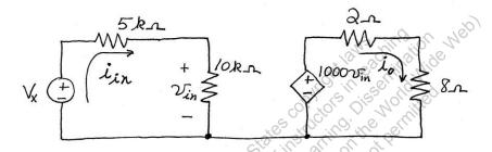
Applying Ohm's law and KVL to the right-hand loop we have  $1000\nu_{in}=2i_o+8i_o$  from which we determine that  $\nu_{in}=10$  mV. Then,  $i_{in}=\nu_{in}/10^4=1~\mu\text{A}$ , and finally we have  $\nu_{x}=5000i_{in}+10000i_{in}=15$  mV.
