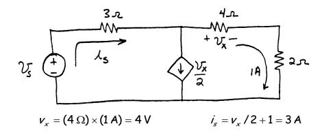
Applying KVL around the outside of the circuit, we have:
