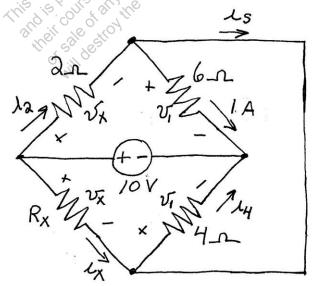
(b)  $R_x$  and the 2- $\Omega$  resistor are in parallel. Also, the 6- $\Omega$  resistor and the the 4- $\Omega$  resistor are in parallel. Thus, the voltages across the parallel elements are the same as labeled in the figure.
