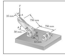
Knowing that  $\theta = 40^{\circ}$  and P = 9 kN, determine (*a*) the smallest allowable diameter of the pin at *B* if the average shearing stress in the pin is not to exceed 120 MPa, (*b*) the corresponding average bearing stress in member *AB* at *B*, (*c*) the corresponding average bearing stress in each of the support brackets at *B*.
