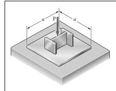
An axial load **P** is supported by a short W8 × 40 column of crosssectional area A = 11.7 in.<sup>2</sup> and is distributed to a concrete foundation by a square plate as shown. Knowing that the average normal stress in the column must not exceed 30 ksi and that the bearing stress on the concrete foundation must not exceed 3.0 ksi, determine the side *a* of the plate that will provide the most economical and safe design.
