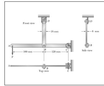
Solve Prob. 1.51, assuming that the structure has been redesigned to use 12-mm-diameter pins at B and D and no other change has been made.
