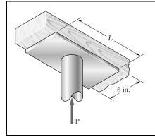
The axial force in the column supporting the timber beam shown is P = 20 kips. Determine the smallest allowable length *L* of the bearing plate if the bearing stress in the timber is not to exceed 400 psi.
