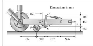
An aircraft tow bar is positioned by means of a single hydraulic cylinder connected by a 25-mm-diameter steel rod to two identical arm-and-wheel units *DEF*. The mass of the entire tow bar is 200 kg, and its center of gravity is located at *G*. For the position shown, determine the normal stress in the rod.
