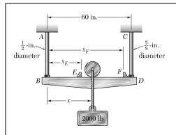
The 2000-lb load can be moved along the beam *BD* to any position between stops at *E* and *F*. Knowing that  $\sigma_{all} = 6$  ksi for the steel used in rods *AB* and *CD*, determine where the stops should be placed if the permitted motion of the load is to be as large as possible.
