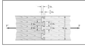
Two wooden planks, each  $\frac{1}{2}$  in. thick and 9 in. wide, are joined by the dry mortise joint shown. Knowing that the wood used shears off along its grain when the average shearing stress reaches 1.20 ksi, determine the magnitude *P* of the axial load that will cause the joint to fail.
