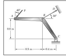
Member *ABC*, which is supported by a pin and bracket at *C* and a cable *BD*, was designed to support the 16-kN load **P** as shown. Knowing that the ultimate load for cable *BD* is 100 kN, determine the factor of safety with respect to cable failure.
