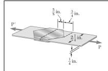
Two plates, each  $\frac{1}{8}$  in. thick, are used to splice a plastic strip as shown. Knowing that the ultimate shearing stress of the bonding between the surface is 130 psi, determine the factor of safety with respect to shear when P = 325 lb.
