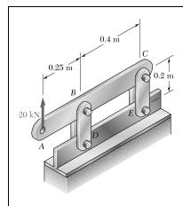
For the assembly and loading of Prob. 1.7, determine (*a*) the average shearing stress in the pin at *B*, (*b*) the average bearing stress at *B* in member *BD*, (*c*) the average bearing stress at *B* in member *ABC*, knowing that this member has a  $10 \times 50$ -mm uniform rectangular cross section.
