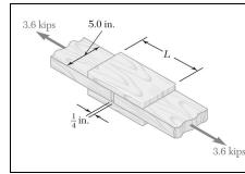
Two wooden members shown, which support a 3.6 kip load, are joined by plywood splices fully glued on the surfaces in contact. The ultimate shearing stress in the glue is 360 psi and the clearance between the members is  $\frac{1}{4}$  in. Determine the required length L of each splice if a factor of safety of 2.75 is to be achieved.
