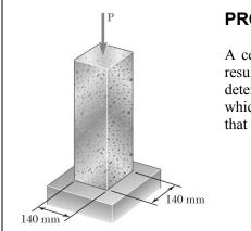
A centric load **P** is applied to the granite block shown. Knowing that the resulting maximum value of the shearing stress in the block is 18 MPa, determine (a) the magnitude of **P**, (b) the orientation of the surface on which the maximum shearing stress occurs, (c) the normal stress exerted on that surface, (d) the maximum value of the normal stress in the block.
