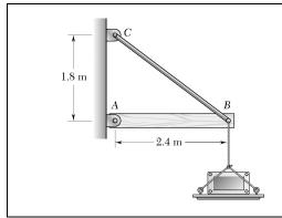
A 40-kg platform is attached to the end *B* of a 50-kg wooden beam *AB*, which is supported as shown by a pin at *A* and by a slender steel rod *BC* with a 12-kN ultimate load. (*a*) Using the Load and Resistance Factor Design method with a resistance factor  $\phi = 0.90$  and load factors  $\gamma_D = 1.25$  and  $\gamma_L = 1.6$ , determine the largest load that can be safely placed on the platform. (*b*) What is the corresponding conventional factor of safety for rod *BC*?
