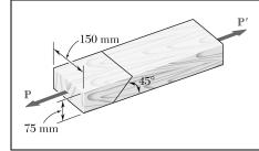
Two wooden members of uniform rectangular cross section are joined by the simple glued scarf splice shown. Knowing that P = 11 kN, determine the normal and shearing stresses in the glued splice.
