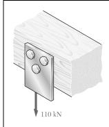
Three steel bolts are to be used to attach the steel plate shown to a wooden beam. Knowing that the plate will support a 110-kN load, that the ultimate shearing stress for the steel used is 360 MPa, and that a factor of safety of 3.35 is desired, determine the required diameter of the bolts.
