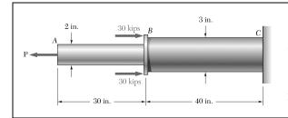
Two solid cylindrical rods AB and BC are welded together at B and loaded as shown. Determine the magnitude of the force **P** for which the tensile stress in rod AB is twice the magnitude of the compressive stress in rod BC.
