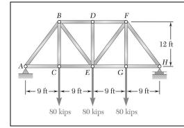
For the Pratt bridge truss and loading shown, determine the average normal stress in member BE, knowing that the cross-sectional area of that member is 5.87 in<sup>2</sup>.
