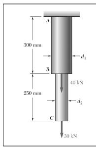
Two solid cylindrical rods *AB* and *BC* are welded together at *B* and loaded as shown. Knowing that  $d_1 = 50 \text{ mm}$  and  $d_2 = 30 \text{ mm}$ , find the average normal stress at the midsection of (*a*) rod *AB*, (*b*) rod *BC*.
