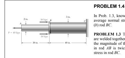
In Prob. 1.3, knowing that P = 40 kips, determine the average normal stress at the midsection of (a) rod AB, (b) rod BC.
