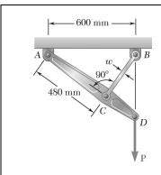
Link *BC* is 6 mm thick and is made of a steel with a 450-MPa ultimate strength in tension. What should be its width w if the structure shown is being designed to support a 20-kN load **P** with a factor of safety of 3?
