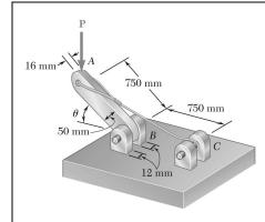
Determine the largest load **P** which may be applied at *A* when  $\theta = 60^{\circ}$ , knowing that the average shearing stress in the 10-mm-diameter pin at *B* must not exceed 120 MPa and that the average bearing stress in member *AB* and in the bracket at *B* must not exceed 90 MPa.
