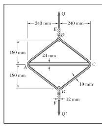
A steel loop *ABCD* of length 1.2 m and of 10-mm diameter is placed as shown around a 24-mm-diameter aluminum rod *AC*. Cables *BE* and *DF*, each of 12-mm diameter, are used to apply the load  $\mathbf{Q}$ . Knowing that the ultimate strength of the steel used for the loop and the cables is 480 MPa and that the ultimate strength of the aluminum used for the rod is 260 MPa, determine the largest load  $\mathbf{Q}$  that can be applied if an overall factor of safety of 3 is desired.
