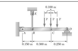
Three forces, each of magnitude P = 4 kN, are applied to the mechanism shown. Determine the cross-sectional area of the uniform portion of rod *BE* for which the normal stress in that portion is +100 MPa.
