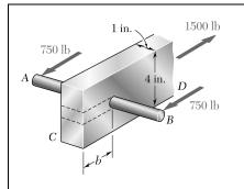
A  $\frac{5}{8}$ -in.-diameter steel rod *AB* is fitted to a round hole near end *C* of the wooden member *CD*. For the loading shown, determine (*a*) the maximum average normal stress in the wood, (*b*) the distance *b* for which the average shearing stress is 100 psi on the surfaces indicated by the dashed lines, (*c*) the average bearing stress on the wood.
