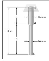
Two brass rods AB and BC, each of uniform diameter, will be brazed together at *B* to form a nonuniform rod of total length 100 m, which will be suspended from a support at *A* as shown. Knowing that the density of brass is 8470 kg/m<sup>3</sup>, determine (*a*) the length of rod *AB* for which the maximum normal stress in *ABC* is minimum, (*b*) the corresponding value of the maximum normal stress.
