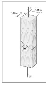
The 1.4-kip load  $\mathbf{P}$  is supported by two wooden members of uniform cross section that are joined by the simple glued scarf splice shown. Determine the normal and shearing stresses in the glued splice.
