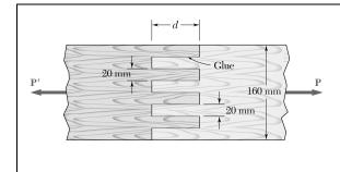
Two wooden planks, each 22 mm thick and 160 mm wide, are joined by the glued mortise joint shown. Knowing that the joint will fail when the average shearing stress in the glue reaches 820 kPa, determine the smallest allowable length d of the cuts if the joint is to withstand an axial load of magnitude P = 7.6 kN.
