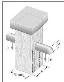
For the support of Prob. 1.45, knowing that the diameter of the pin is d = 16 mm and that the magnitude of the load is P = 20 kN, determine (*a*) the factor of safety for the pin, (*b*) the required values of *b* and *c* if the factor of safety for the wooden members is the same as that found in part *a* for the pin.
