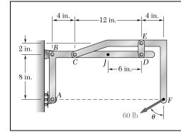
Knowing that the link *DE* is  $\frac{1}{8}$  in. thick and 1 in. wide, determine the normal stress in the central portion of that link when (*a*)  $\theta = 0^{\circ}$ , (*b*)  $\theta = 90^{\circ}$ .
