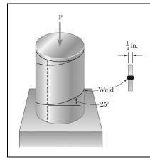
A steel pipe of 12-in. outer diameter is fabricated from  $\frac{1}{4}$ -in.-thick plate by welding along a helix that forms an angle of 25° with a plane perpendicular to the axis of the pipe. Knowing that the maximum allowable normal and shearing stresses in the directions respectively normal and tangential to the weld are  $\sigma = 12$  ksi and  $\tau = 7.2$  ksi, determine the magnitude P of the largest axial force that can be applied to the pipe.
