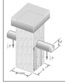
A load **P** is supported as shown by a steel pin that has been inserted in a short wooden member hanging from the ceiling. The ultimate strength of the wood used is 60 MPa in tension and 7.5 MPa in shear, while the ultimate strength of the steel is 145 MPa in shear. Knowing that b = 40 mm, c = 55 mm, and d = 12 mm, determine the load **P** if an overall factor of safety of 3.2 is desired.
