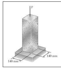
A 1060-kN load **P** is applied to the granite block shown. Determine the resulting maximum value of (a) the normal stress, (b) the shearing stress. Specify the orientation of the plane on which each of these maximum values occurs.
