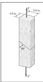
Two wooden members of uniform cross section are joined by the simple scarf splice shown. Knowing that the maximum allowable tensile stress in the glued splice is 75 psi, determine (a) the largest load **P** that can be safely supported, (b) the corresponding shearing stress in the splice.
