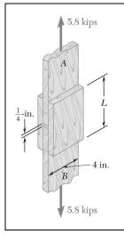
The wooden members A and B are to be joined by plywood splice plates, that will be fully glued on the surfaces in contact. As part of the design of the joint, and knowing that the clearance between the ends of the members is to be  $\frac{1}{4}$  in., determine the smallest allowable length L if the average shearing stress in the glue is not to exceed 120 psi.
