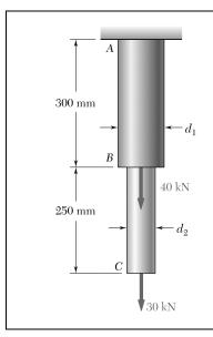
Two solid cylindrical rods *AB* and *BC* are welded together at *B* and loaded as shown. Knowing that the average normal stress must not exceed 175 MPa in rod *AB* and 150 MPa in rod *BC*, determine the smallest allowable values of  $d_1$  and  $d_2$ .
