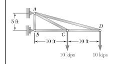
A  $\frac{3}{4}$ -in.-diameter rod made of the same material as rods AC and AD in the truss shown was tested to failure and an ultimate load of 29 kips was recorded. Using a factor of safety of 3.0, determine the required diameter (a) of rod AC, (b) of rod AD.
