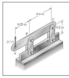
Each of the four vertical links has an  $8 \times 36$ -mm uniform rectangular cross section and each of the four pins has a 16-mm diameter. Determine the maximum value of the average normal stress in the links connecting (*a*) points *B* and *D*, (*b*) points *C* and *E*.
