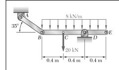
Link AB is to be made of a steel for which the ultimate normal stress is 450 MPa. Determine the cross-sectional area for AB for which the factor of safety will be 3.50. Assume that the link will be adequately reinforced around the pins at A and B.
