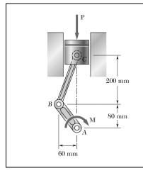
A couple **M** of magnitude 1500 N  $\cdot$  m is applied to the crank of an engine. For the position shown, determine (*a*) the force **P** required to hold the engine system in equilibrium, (*b*) the average normal stress in the connecting rod *BC*, which has a 450-mm<sup>2</sup> uniform cross section.
