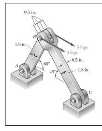
For the assembly and loading of Prob. 1.60, determine (a) the average shearing stress in the pin at C, (b) the average bearing stress at C in member BC, (c) the average bearing stress at B in member BC.
