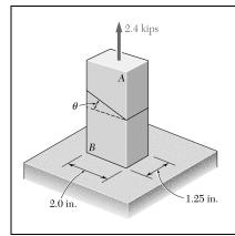
The two portions of member *AB* are glued together along a plane forming an angle  $\theta$  with the horizontal. Knowing that the ultimate stress for the glued joint is 2.5 ksi in tension and 1.3 ksi in shear, determine the range of values of  $\theta$  for which the factor of safety of the members is at least 3.0.
