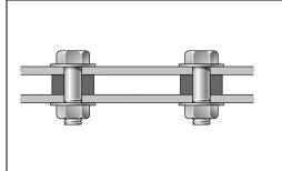
Two steel plates are to be held together by means of 16-mmdiameter high-strength steel bolts fitting snugly inside cylindrical brass spacers. Knowing that the average normal stress must not exceed 200 MPa in the bolts and 130 MPa in the spacers, determine the outer diameter of the spacers that yields the most economical and safe design.
