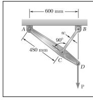
Link *BC* is 6 mm thick, has a width w = 25 mm, and is made of a steel with a 480-MPa ultimate strength in tension. What was the safety factor used if the structure shown was designed to support a 16-kN load **P**?
