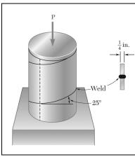
A steel pipe of 12-in. outer diameter is fabricated from  $\frac{1}{4}$ -in.-thick plate by welding along a helix that forms an angle of 25° with a plane perpendicular to the axis of the pipe. Knowing that a 66 kip axial force **P** is applied to the pipe, determine the normal and shearing stresses in directions respectively normal and tangential to the weld.
