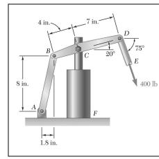
The hydraulic cylinder *CF*, which partially controls the position of rod *DE*, has been locked in the position shown. Member *BD* is  $\frac{5}{8}$  in. thick and is connected to the vertical rod by a  $\frac{3}{8}$ -in.-diameter bolt. Determine (*a*) the average shearing stress in the bolt, (*b*) the bearing stress at *C* in member *BD*.
