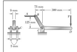
Knowing that a force **P** of magnitude 750 N is applied to the pedal shown, determine (*a*) the diameter of the pin at *C* for which the average shearing stress in the pin is 40 MPa, (*b*) the corresponding bearing stress in the pedal at *C*, (*c*) the corresponding bearing stress in each support bracket at *C*.
