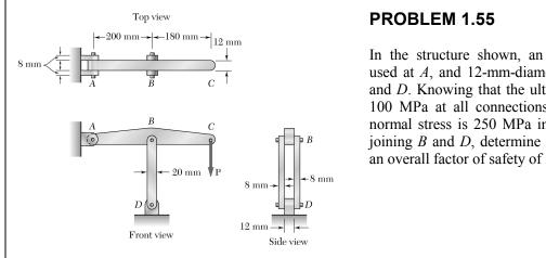
In the structure shown, an 8-mm-diameter pin is used at A, and 12-mm-diameter pins are used at B and D. Knowing that the ultimate shearing stress is 100 MPa at all connections and that the ultimate normal stress is 250 MPa in each of the two links joining B and D, determine the allowable load  $\mathbf{P}$  if an overall factor of safety of 3.0 is desired.
