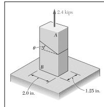
The two portions of member *AB* are glued together along a plane forming an angle  $\theta$  with the horizontal. Knowing that the ultimate stress for the glued joint is 2.5 ksi in tension and 1.3 ksi in shear, determine (*a*) the value of  $\theta$  for which the factor of safety of the member is maximum, (*b*) the corresponding value of the factor of safety. (*Hint:* Equate the expressions obtained for the factors of safety with respect to normal stress and shear.)
