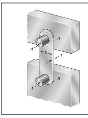
Link AB, of width b = 50 mm and thickness t = 6 mm, is used to support the end of a horizontal beam. Knowing that the average normal stress in the link is -140 MPa, and that the average shearing stress in each of the two pins is 80 MPa, determine (*a*) the diameter *d* of the pins, (*b*) the average bearing stress in the link.
