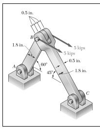
Two horizontal 5-kip forces are applied to pin B of the assembly shown. Knowing that a pin of 0.8-in. diameter is used at each connection, determine the maximum value of the average normal stress (a) in link AB, (b) in link BC.
