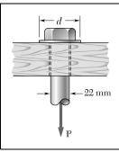
The load **P** applied to a steel rod is distributed to a timber support by an annular washer. The diameter of the rod is 22 mm and the inner diameter of the washer is 25 mm, which is slightly larger than the diameter of the hole. Determine the smallest allowable outer diameter d of the washer, knowing that the axial normal stress in the steel rod is 35 MPa and that the average bearing stress between the washer and the timber must not exceed 5 MPa.
