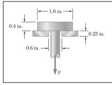
A load **P** is applied to a steel rod supported as shown by an aluminum plate into which a 0.6-in.-diameter hole has been drilled. Knowing that the shearing stress must not exceed 18 ksi in the steel rod and 10 ksi in the aluminum plate, determine the largest load **P** that can be applied to the rod.
