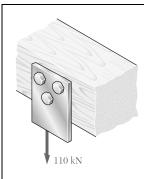
Three 18-mm-diameter steel bolts are to be used to attach the steel plate shown to a wooden beam. Knowing that the plate will support a 110-kN load and that the ultimate shearing stress for the steel used is 360 MPa, determine the factor of safety for this design.
