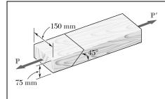
Two wooden members of uniform rectangular cross section are joined by the simple glued scarf splice shown. Knowing that the maximum allowable shearing stress in the glued splice is 620 kPa, determine (a) the largest load **P** that can be safely applied, (b) the corresponding tensile stress in the splice.
