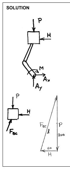
Use piston, rod, and crank together as free body. Add wall reaction H and bearing reactions  $A_x$  and  $A_y$ .
