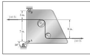
Link AC has a uniform rectangular cross section  $\frac{1}{16}$  in. thick and  $\frac{1}{4}$  in. wide. Determine the normal stress in the central portion of the link.
