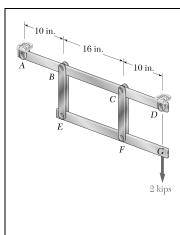
Solve Prob. 1.53, assuming that the pins at *C* and *F* have been replaced by pins with a  $\frac{3}{4}$ -in diameter.
