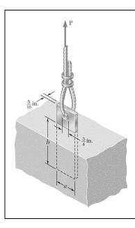
Determine the factor of safety for the cable anchor in Prob. 1.49 when P = 3 kips, knowing that a = 2 in. and b = 7.5 in.
