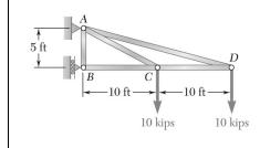
In the truss shown, members AC and AD consist of rods made of the same metal alloy. Knowing that AC is of 1-in. diameter and that the ultimate load for that rod is 75 kips, determine (a) the factor of safety for AC, (b) the required diameter of AD if it is desired that both rods have the same factor of safety.
