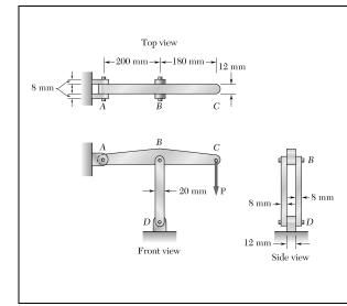
In an alternative design for the structure of Prob. 1.55, a pin of 10-mm-diameter is to be used at A. Assuming that all other specifications remain unchanged, determine the allowable load **P** if an overall factor of safety of 3.0 is desired.
