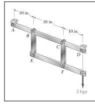
Each of the two vertical links *CF* connecting the two horizontal members *AD* and *EG* has a uniform rectangular cross section  $\frac{1}{4}$  in. thick and 1 in. wide, and is made of a steel with an ultimate strength in tension of 60 ksi. The pins at *C* and *F* each have a  $\frac{1}{2}$ -in. diameter and are made of a steel with an ultimate strength in shear of 25 ksi. Determine the overall factor of safety for the links *CF* and the pins connecting them to the horizontal members.
