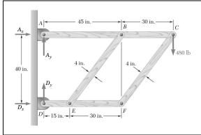
The frame shown consists of *four* wooden members, *ABC*, *DEF*, *BE*, and *CF*. Knowing that each member has a  $2 \times 4$ -in. rectangular cross section and that each pin has a 1/2-in. diameter, determine the maximum value of the average normal stress (*a*) in member *BE*, (*b*) in member *CF*.
