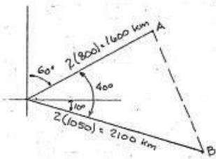
$$\begin{aligned}(AB)^2 &= 1600^2 + 2100^2 - \\&\quad - 2(1600)(2100)\cos 40^\circ \\&= 1350 \text{ km}\end{aligned}$$
