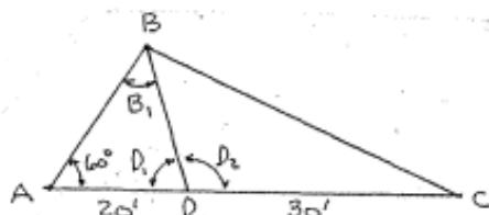
$$\frac{20}{\sin B_1} = \frac{26}{\sin 60^\circ} \rightarrow \therefore B_1 = 41.77^\circ$$
