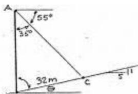
$$\begin{aligned}\theta &= \tan^{-1}(1/5) \\&= 11.31^\circ \\< \text{CBA} &= 90 - 11.31 \\&= 78.69^\circ \\< \text{C} &= 180 - 78.69 - 35 = 66.31^\circ \\ \frac{AB}{\sin 66.31^\circ} &= \frac{32}{\sin 35^\circ} \rightarrow AB = 51.1 \text{ m}\end{aligned}$$
