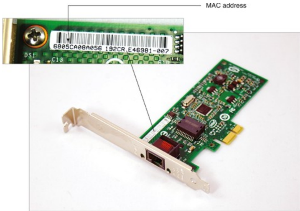
Figure 3: This Gigabit Ethernet adapter by Intel uses a PCIe x1 slot
